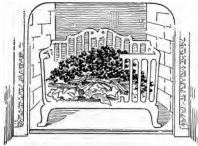
FIG. 58. — The difference in the kindling temperature of paper, wood, and coal is utilized in building a coal fire.
